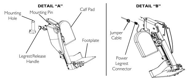
FIGURE 6.22 Installing/Removing the Power Elevating Legrests
